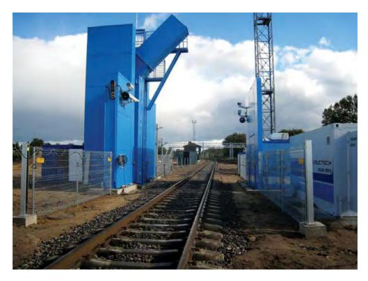
7.82 A further example of a Nuctech scanner with an energy level ranging from 1.5MeV to 6MeV that is used for "inspecting cars, cargo containers, empty containers, container trucks at seaports, border crossings, airports" is shown below 98:
