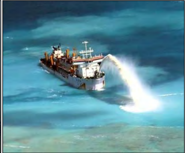
Figure 16: Trailing Suction Hopper Dredge (Annex 792)
